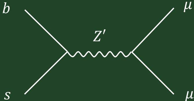
$$C_9^{NP} \sim -0.7 \times \left( \frac{500 \text{ GeV}}{m_{Z'}} \right)^2 \left( \frac{g_{\mu\mu}^V \cdot g_{bs}^L}{0.0003} \right)$$
